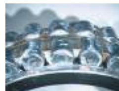
Photo. 6.2 Filling grease into cylindrical roller bearing
