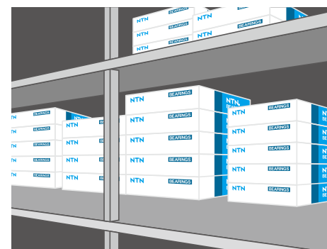
Fig. 15.4 Storing one-bearing boxes on a shelf
