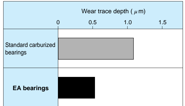
Fig.8 Results of wear test using NTN test unit
