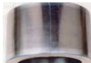
Outer ring cracking
