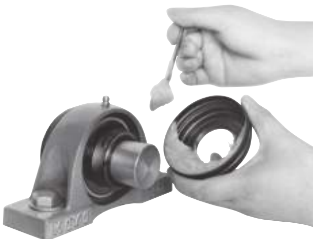
Fig. 14.11 Packing grease in internal space and seal lip of cover
