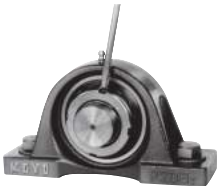
Fig. 14.8 Bending outer tab of washer (Locking locknut)
