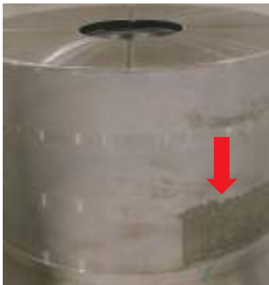
① Flaking of cross raceway surface
