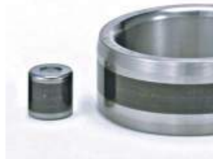
Fig. 4-2 Electric pitting generated on general purpose bearings (pits)
