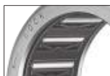
The mounted clutch engages when the housing is rotated relative to the shaft in the direction of the arrow marking (← LOCK) stamped on the cup.
