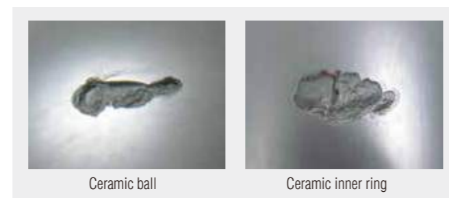
Fig. 6 Flaking on ceramic ball and inner ring
