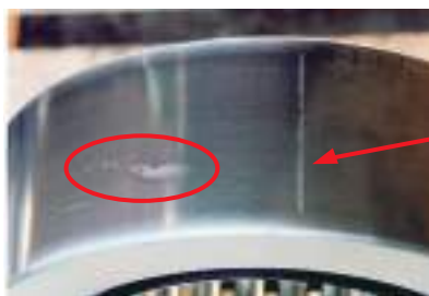
Brinelling on outer ring O.D.
