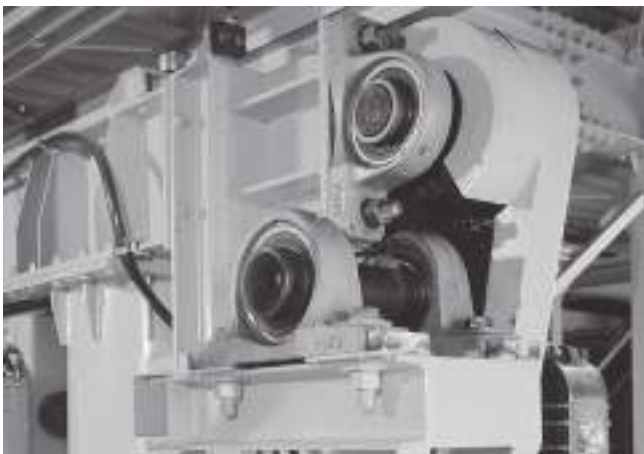
Mast driving system
