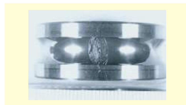
Fig. 1-12 Ceramic inner ring damaged by dynamic strength test
