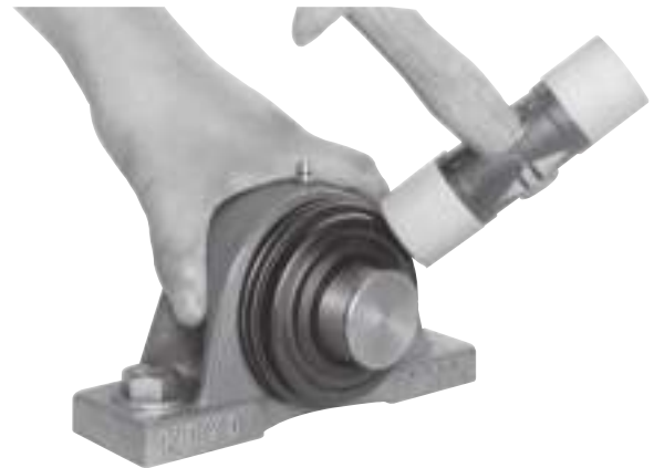
Fig. 14.12 Installing steel plate cover
