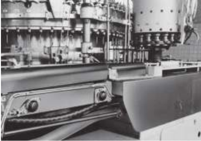
Bottle filling line conveyor
