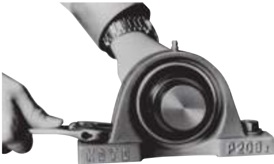
Fig. 14.4 Fixing insert bearing unit to base
