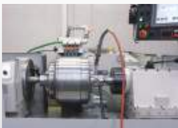
Mounting the regrinding jig and bearing assembly to the cylindrical grinder
