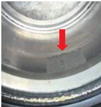
② Flaking of bearing cup raceway surface
