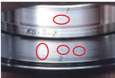
Brinelling on raceway surface of outer ring
