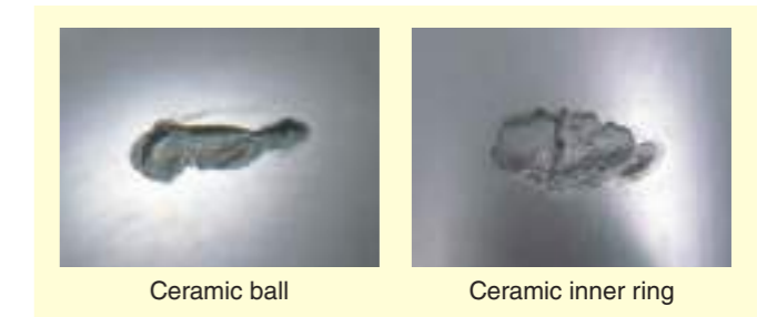
Fig. 1-5 Flaking on ceramic ball and inner ring
