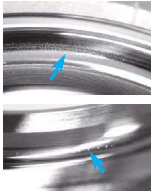
Fig. 1.2 Example of biting flaws formed in raceway because of entry of foreign matter
