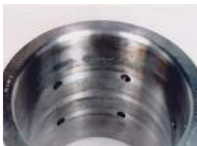
Fretting on bore surface of inner ring
