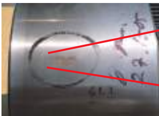
Outside of outer ring's grinding burn
