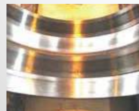
Hardly any indication of rust
