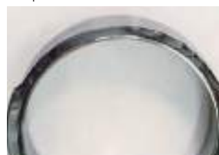
Inner ring cracking
