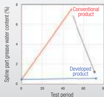
■ Spline muddy water endurance test result
