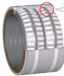
Signs of temperature rise on the roller large end face Scuffing occurrence on the roller large end face
