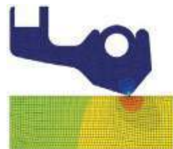
After the shaft is rotated (heat temperature distribution chart)
