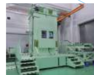
Bearing tester for steel production equipment
